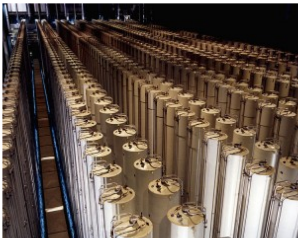
Image: Cascade of gas centrifuges used to produce enriched uranium. (Photo credit: U.S. Department of Energy)
