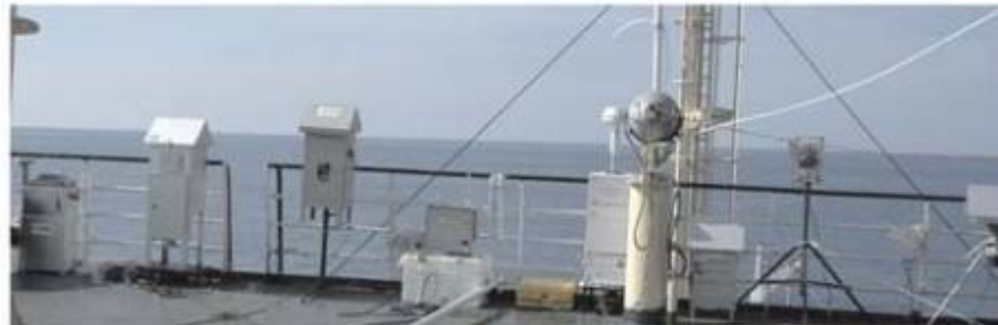
India's on-ship instruments to sample aerosols at sea level.
