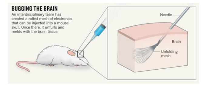
So far, the researchers have implanted meshes consisting of 16 electrical elements into two brain regions of anaesthetized mice, where they were able to both monitor and stimulate individual neurons. The mesh integrates tightly with the neural cells, says Jia Liu, a member of the Harvard team, with no signs of an elevated immune response after five weeks. Neurons "look at this polymer network as friendly, like a scaffold", he says.
