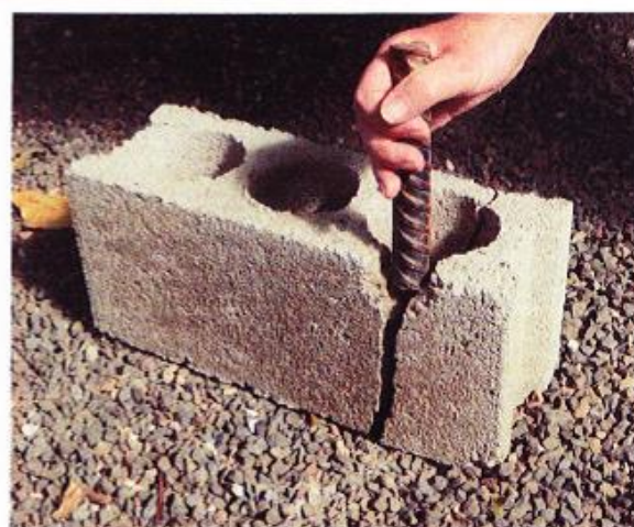
Example of the typical, locally handmade, 600 psi masonry block used for the housing units
