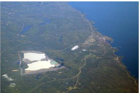
Two views of the "delta" that formed at Silver Bay, Minnesota by Reserve Mining's continuous discharging of taconite tailings directly into Lake Superior. The delta eventually extended 1/3 of a mile from the original shoreline. Reserve Mining attempted to do some remediation, as seen in the second photo that shows some vegetation growing, but the toxins in the underlying sludge will never be fully de-toxified.
