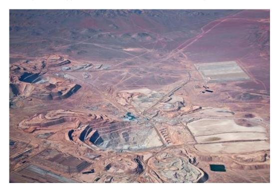
The Escondida mine tailings lagoon above – in Chile's Atacama desert – is the world's largest tailings pond. The tailings are intended to be held in perpetuity behind earthen retaining dams. The straight line at the left of the photo represents the tallest of the surrounding retaining walls, and is 0.6 miles long. NASA satellite photo.
