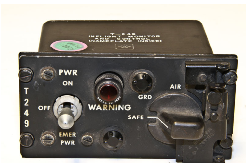
The T-249 switch used to arm nuclear bombs on Strategic Air Command bomber aircraft. Photo courtesy of Glenn's Computer Museum
