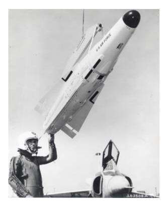
The U.S. Air Force's Falcon (GAR-11) guided nuclear antiaircraft missile with an interceptor in the background. The nuclear Falcon entered the inventory in 1961 as the result of the Air Force's decision to have a nuclear antiaircraft weapon capable of being carried by the F-102 Delta Dagger interceptor. The Falcon's W-54 warhead yielded about one-quarter kiloton.
