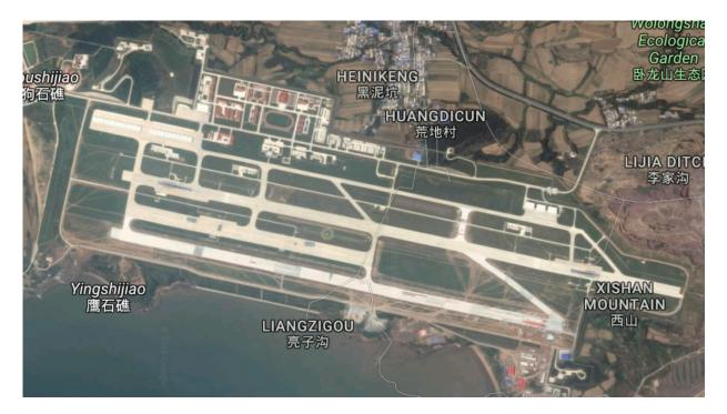
Satellite imagery of Huangdicun Airbase in its entirety, showing the orientation of skiramps, arrestor landing areas, catapults, hangars for J-15 naval strike fighters and support buildings are clearly visible.
