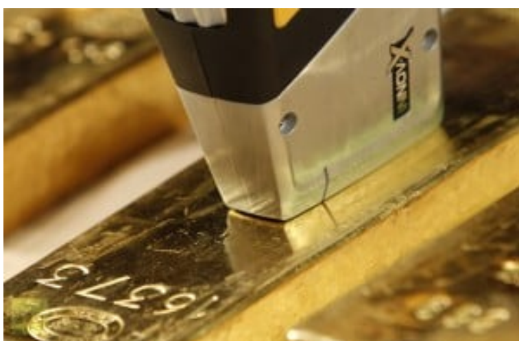
An employee of Deutsche Bundesbank uses a metal analysis device on a gold bar. (Reuters / Lisi Niesner)
