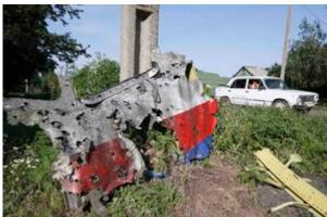
External forces were recorded almost exclusively in the front of the plane, namely the cockpit, and this led to the breakup of the aircraft.
