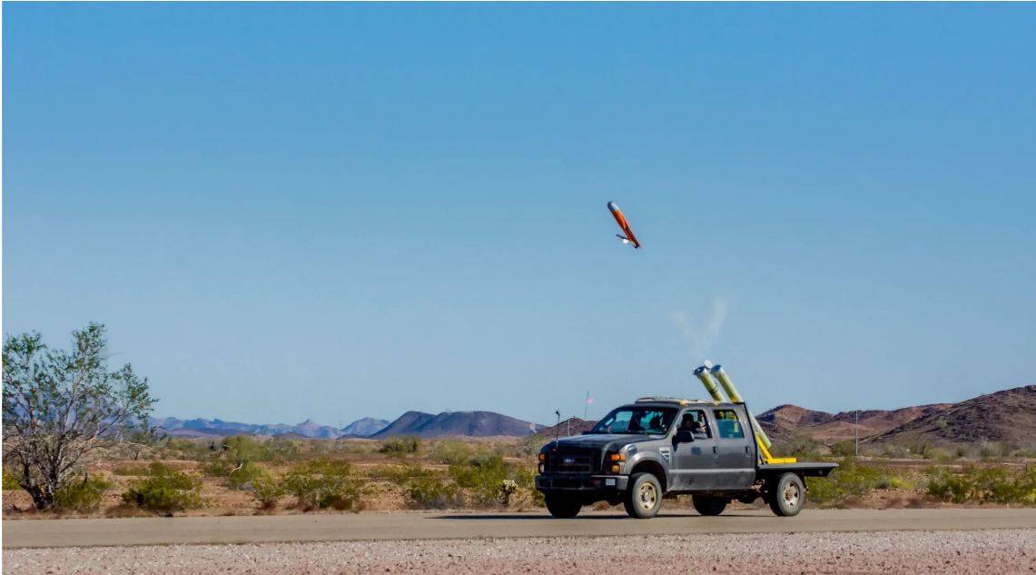
An ALTIUS is launched from an Area-I Pneumatically Integrated Launch System (PILS) during EDGE 21. Area-I photo
