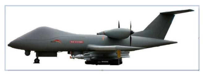
Mantis is closer in appearance to existing armed drones but more advanced in its specification and powered by two Rolls Royce model 250 turboprop engines (see photo). Its first test flight took place in October 2009.
